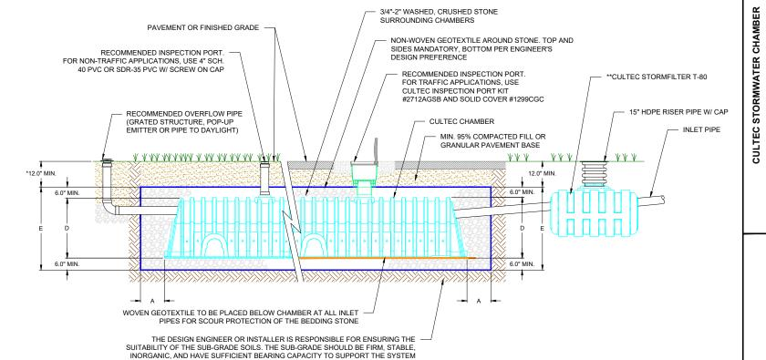
\*FOR NON-TRAFFIC APPLICATIONS, THE DEPTH OF COVER ABOVE THE EMBEDMENT STONE LAYER MAY BE REDUCED TO 6.0"
